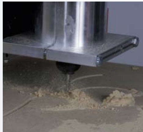
below Fire up and watch the bit cut, note the downcut bit keeps dust to a minimum
