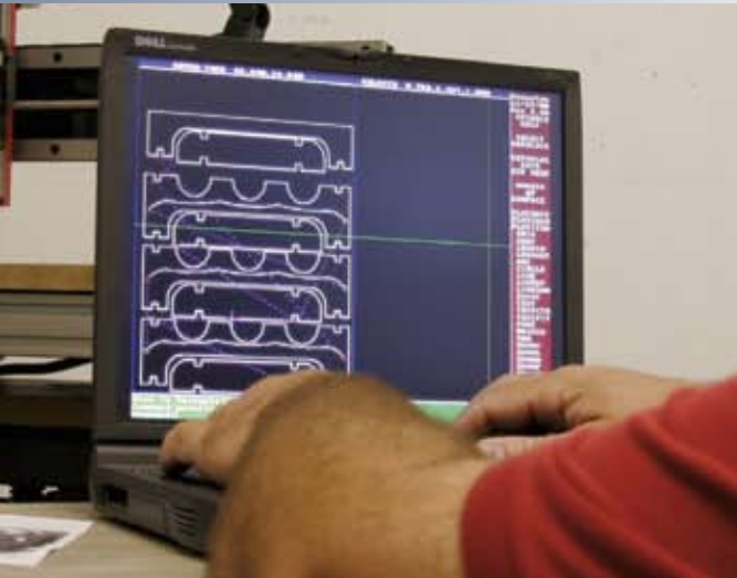
below Once the drawing is imported it is shown on the machine's PC screen
